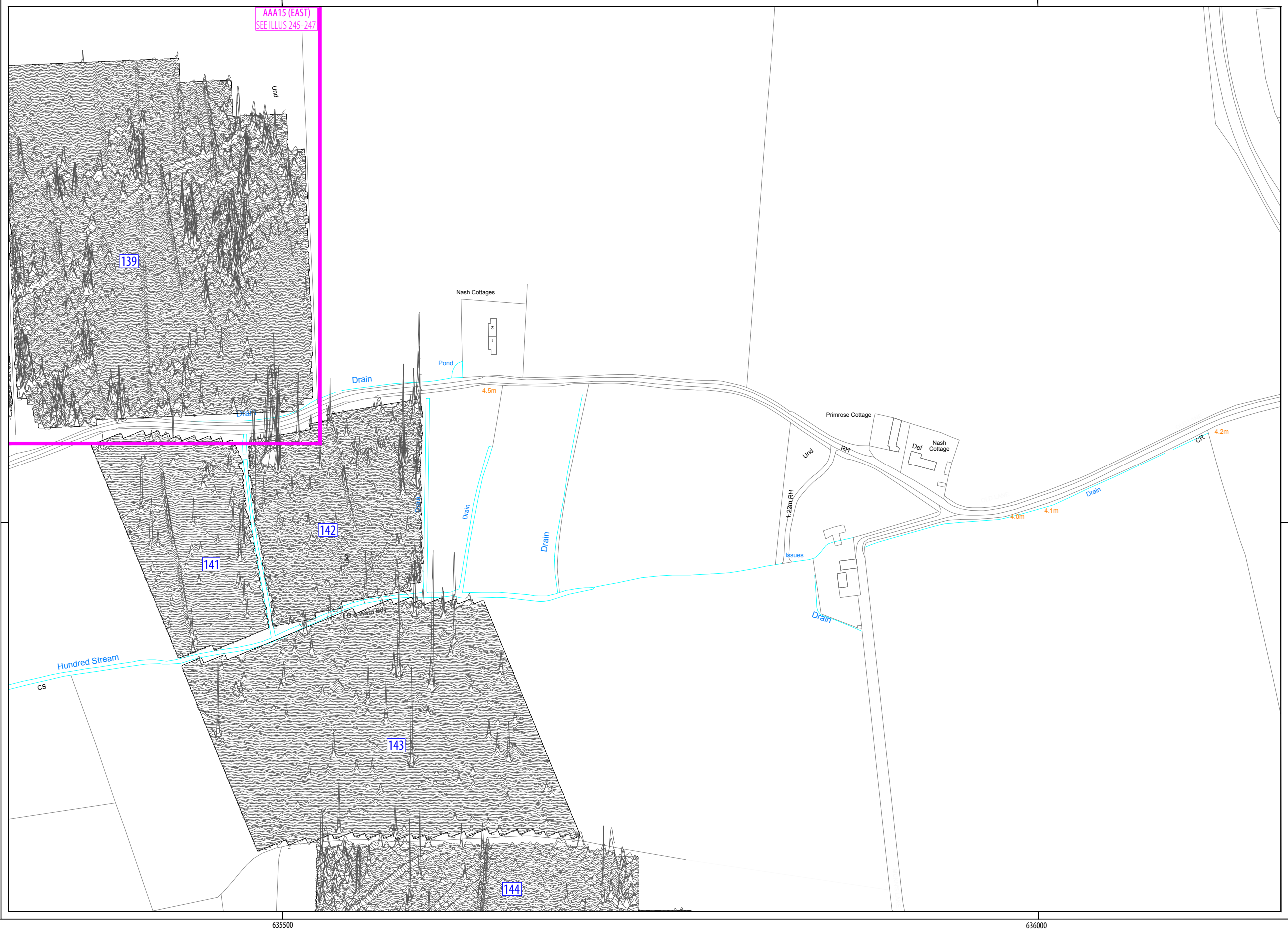
ILLUS 174 XY trace plot of minimally processed of magnetometer data; PAGSA 139-144
